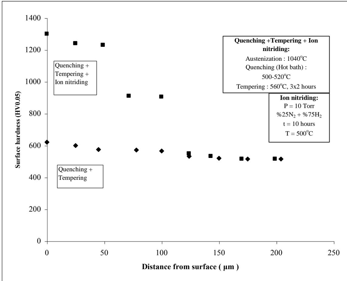
Figure 5. The hardness distributions of quenched and tempered AISI H13 steel and ion nitrided AISI H13 steel distance from the surface to the inside
