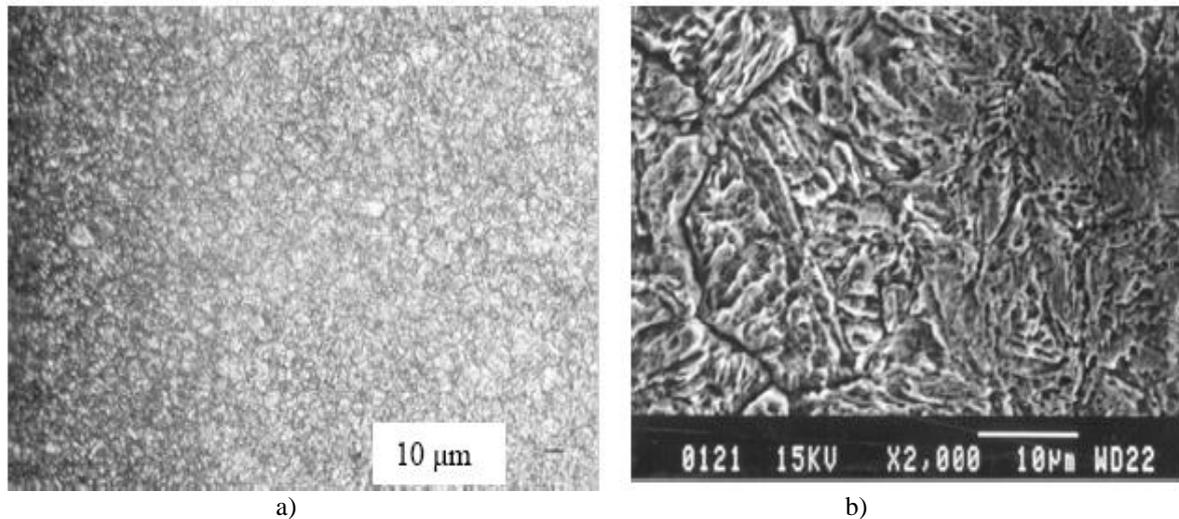
Figure 3. Microstructures of ion nitrided AISI H13 steel; a) Optical microscope, b) Electron microscope (SEM)
