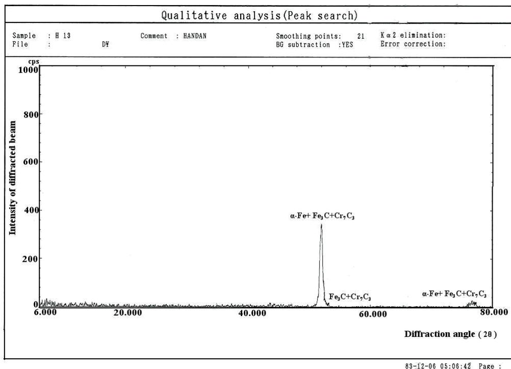
Figure 2. X-Ray diffraction of quenched-tempered AISI H13 steel
