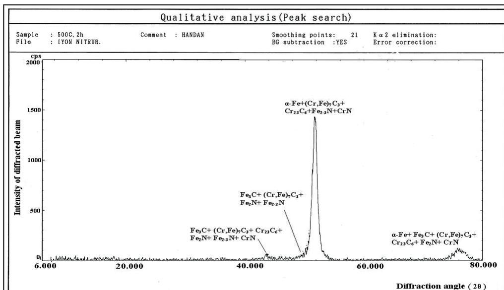
Figure 7. X-ray diffraction analyse of ion nitrided AISI H13 steel (500 °C – 2 hours).
