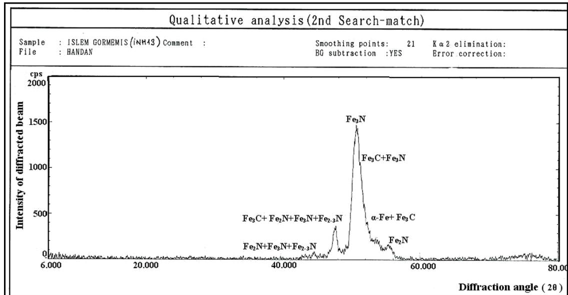
Figure 4. X-Ray diffraction analysis of ion nitrided AISI H13 steel
