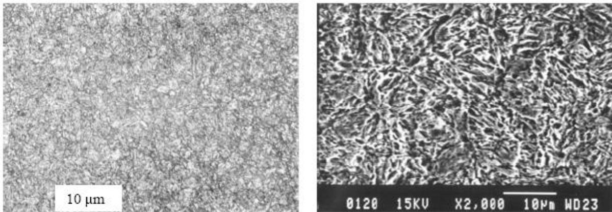
Figure 1. Microstructures of quenched-tempered AISI H13 steel; a) Optical microscope, b) Scanning electron microscope (SEM)
