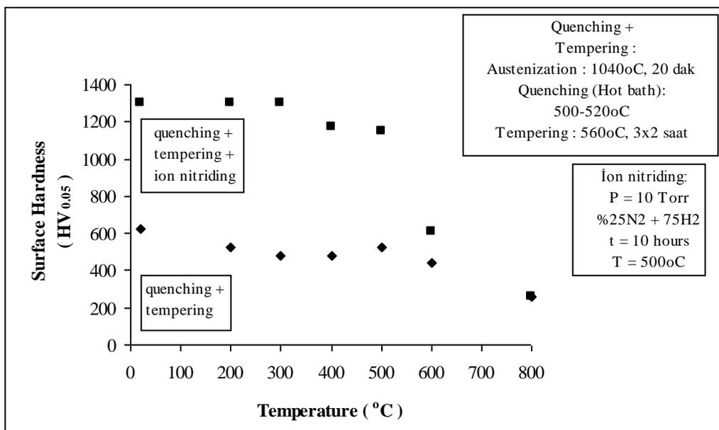
Figure 6. The surface hardness distributions of quenched and tempered AISI H13 steel and ion nitrided AISI H13 steel (20 °, 200 °, 300 °, 400 °, 500 °C – 2 hours).
