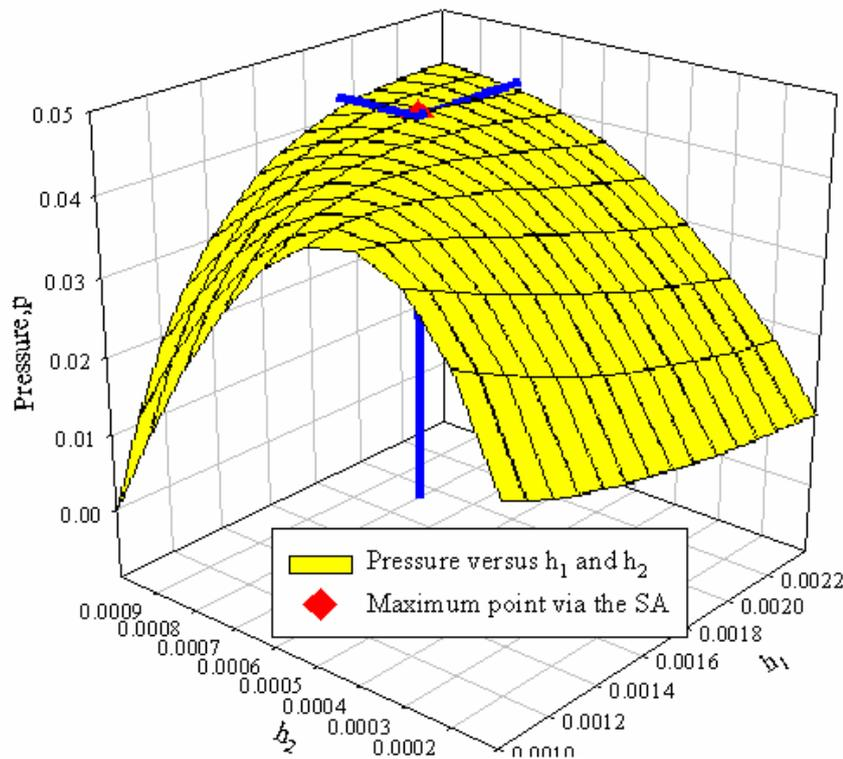
Figure 3. Lubrication pressure profile versus  $h_1$  and  $h_2$
