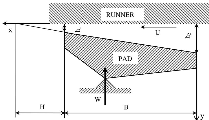
Figure 2. Schematic representation of a single pivoted-pad thrust bearing
