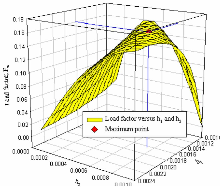
Figure 5. Variation of load factor versus  $h_1$  and  $h_2$
