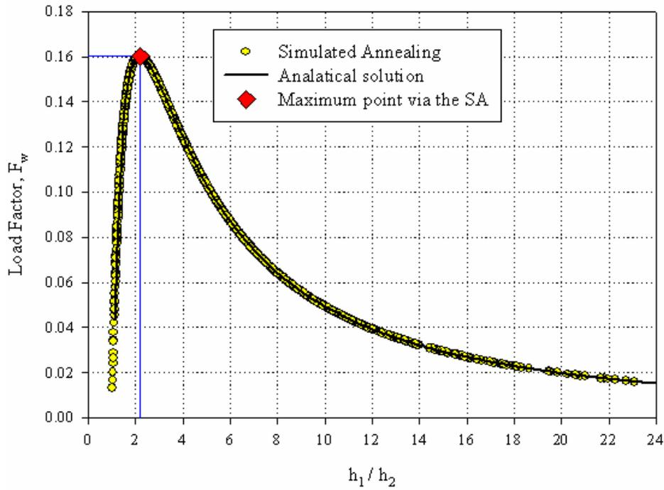
Figure 4. Variation of load factor versus pad inclination,  $h_1 / h_2$
