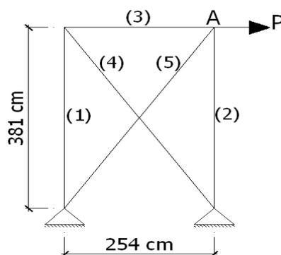
Figure 5. Truss with Double Braced Panel
