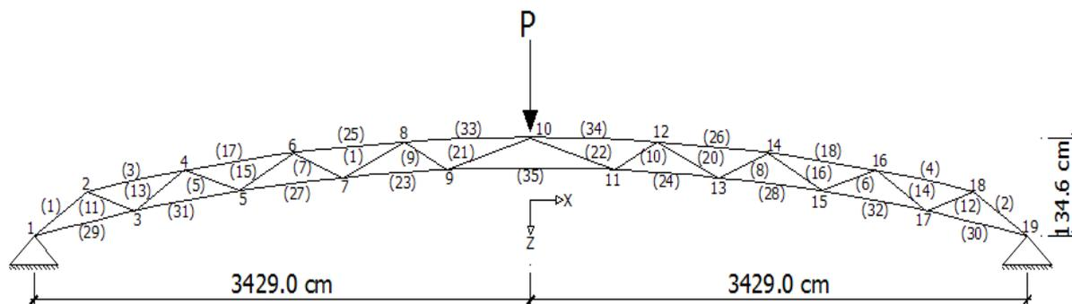
Figure 9. Arch Truss
