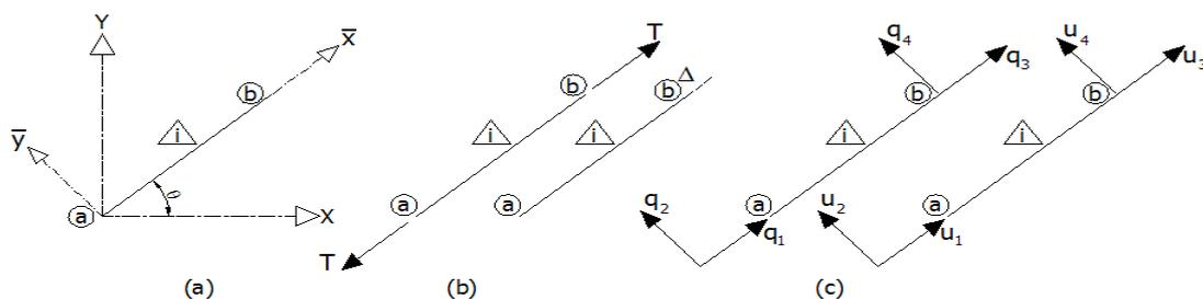
Figure 2. Truss Member: (a) Global and Local Axes, (b) Basic Forces and Displacements, (c) Local Forces and Displacements
