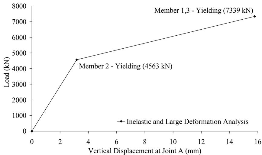
Figure 4. Load-Vertical Displacement of Three-Element Truss
