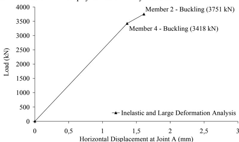
Figure 6. Load–Horizontal Displacement of Truss with Double Braced Panel
