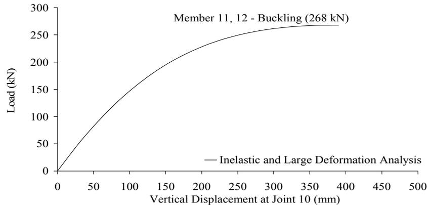
Figure 10. Load–Vertical Displacement of Arch Truss
