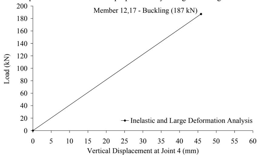
Figure 8. Load – Vertical Displacement of Pratt Truss
