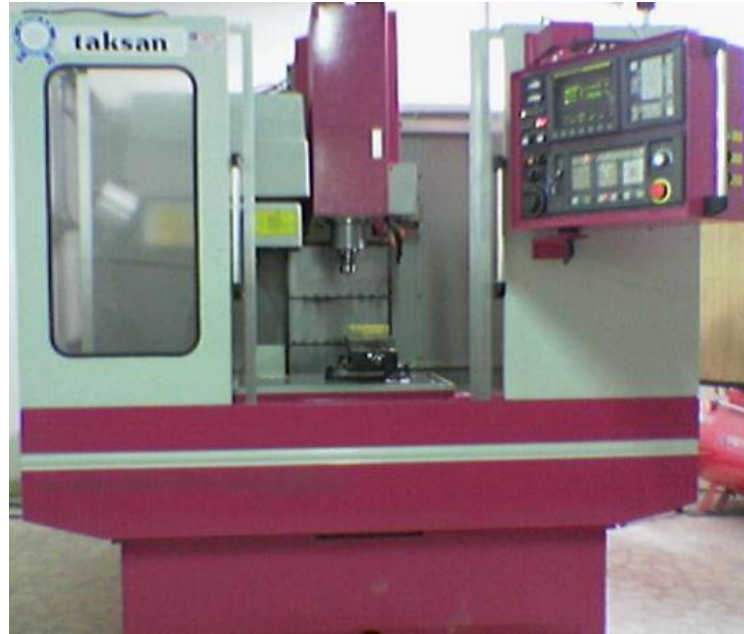
Fig. 2. Taksan TMC500-OM CNC vertical machining centre
