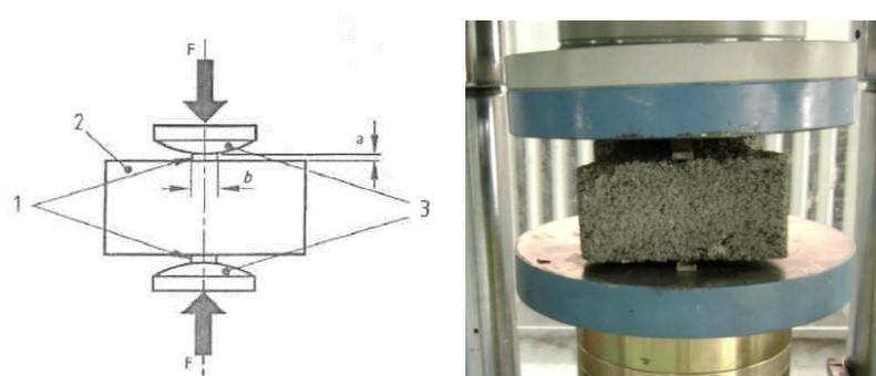
**Figure 1.** Splitting tensile strength test
