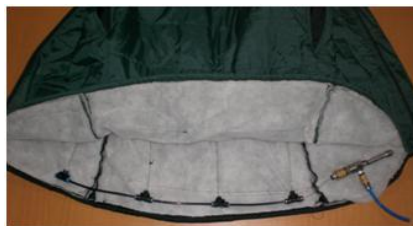
Figure 5. Set pipes and couplings on vest.
