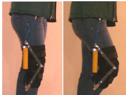
Figure 4. Open and close position of piston mechanism
