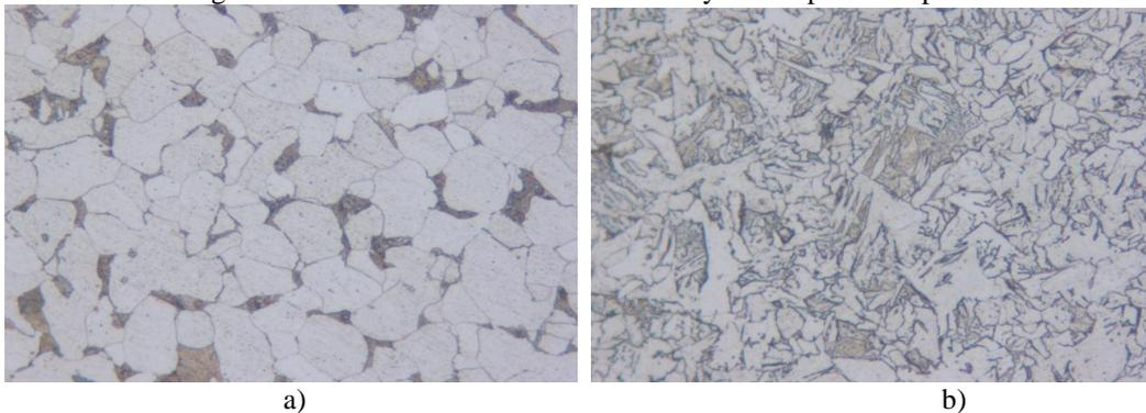
Figure 2. Microstructure images of AISI 1022 steel with 15 ppm boron cooled in a) air and b) water (X500)
