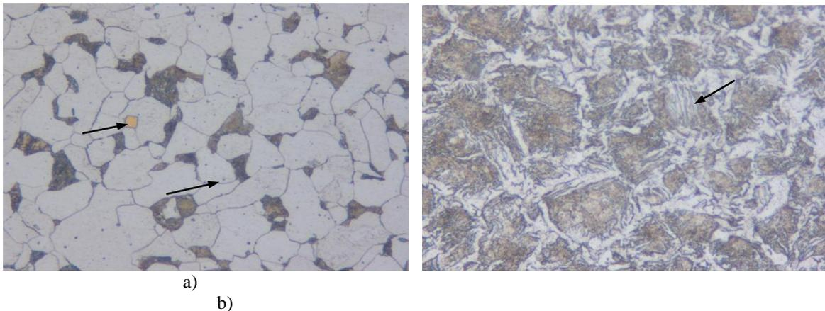
Figure 1. Microstructure images of AISI 1022 steel without boron cooled in a) air and b) water (X500)
