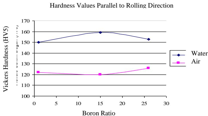
Figure 5. Hardness values of air- and water-cooled AISI 1022 material obtained as parallel to rolling direction
