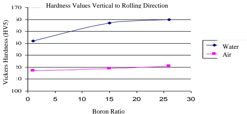
Figure 4. Hardness values of air- and water-cooled AISI 1022 material obtained as vertical to rolling direction
