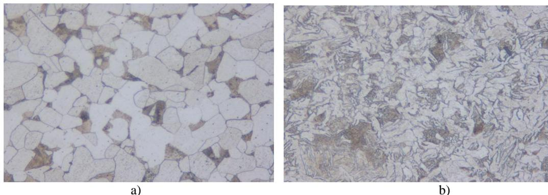
Figure 3. Microstructure images of AISI 1022 steel with 26 ppm boron cooled in a) air and b) water (X500)
