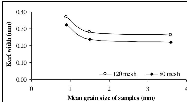
Fig. 5. Effect of the abrasive size on the kerf width of the concrete samples
