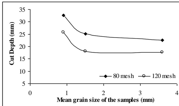
Fig. 4. Effect of the abrasive size on the cut depth of the concrete samples
