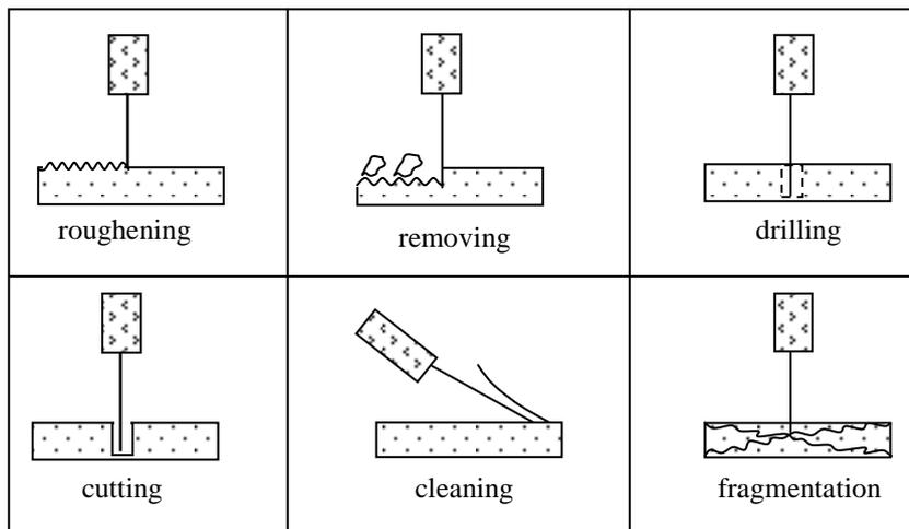
Fig. 1. Cases of application of water jets for concrete processing
