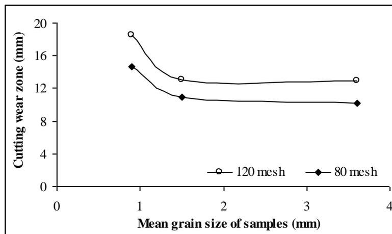
Fig. 6. . Effect of the abrasive size on the cutting wear zone of the concrete samples
