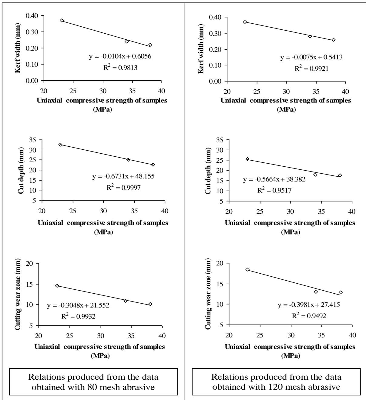
Fig.7. Relation between uniaxial compressive strength of samples and cutting performance (with 80 and 120 mesh abrasive)
