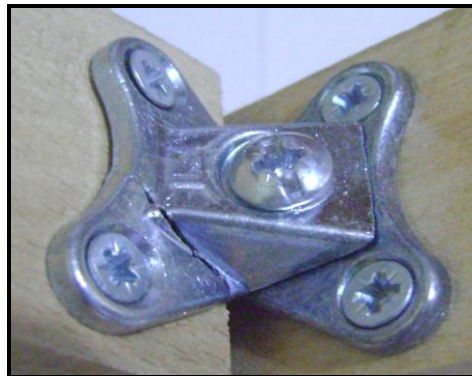
Figure 17. The experimental deformations of Bent Metal “T” Pulling Joint Element
