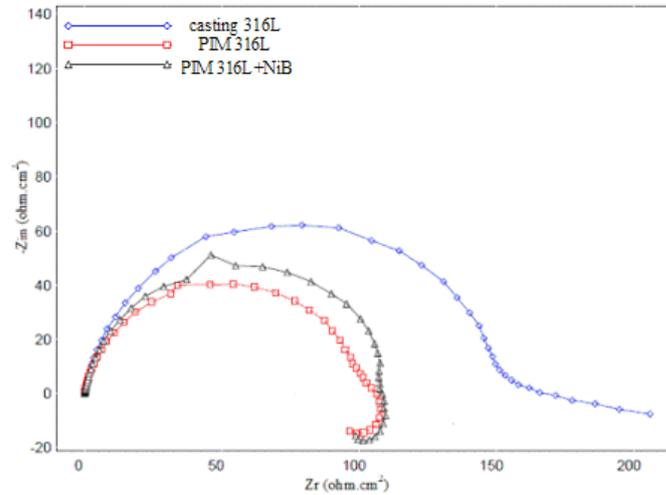
**Figure 4.** Nyquist curves for casting 316L, PIM 316L and PIM 316L+NiB stainless steels in 1M HCl
