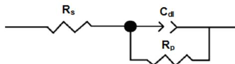
**Figure 3.** Equivalent circuit
