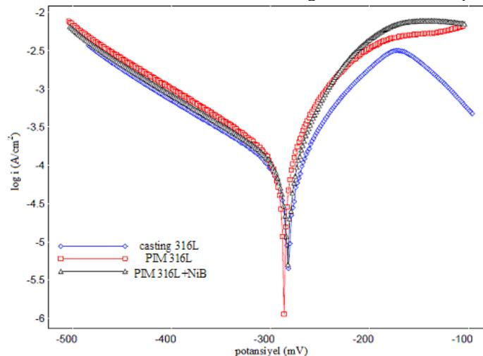
**Figure 1.** Tafel curves for casting 316L, PIM 316L and PIM 316L+NiB stainless steels in 1M HCl
