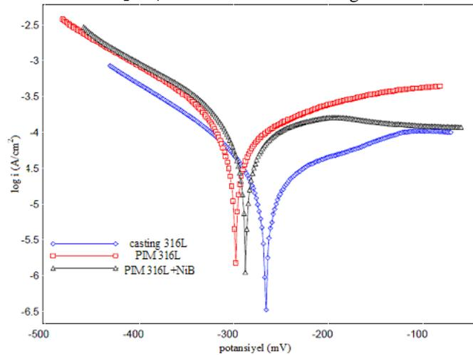
**Figure 2.** Tafel curves for casting 316L, PIM 316L and PIM 316L+NiB stainless steels in 1M H<sub>2</sub>SO<sub>4</sub>
