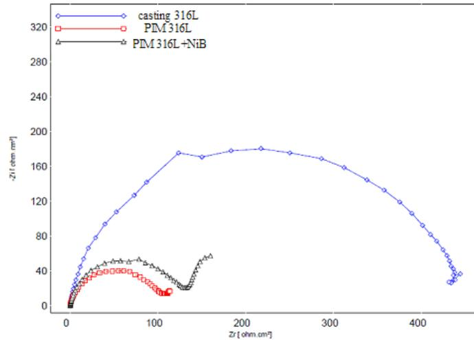
**Figure 5.** Nyquist curves for casting 316L, PIM 316L and PIM 316L+NiB stainless steels in 1M H<sub>2</sub>SO<sub>4</sub>
