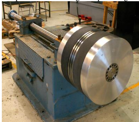
Figure 2 An example of a large size piston and piston rod for a large reciprocating compressor.
