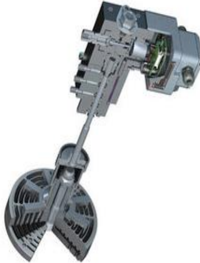
Figure 4 An example of a step-less capacity control for a reciprocating compressor. This complex system is used on a ring type valve in this example. It is recommended for large reciprocating compressors with extended operating times at part-loads.
