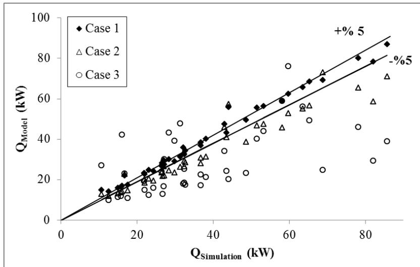
**Figure 3.** Heat capacities obtained from model 1 for different cases
