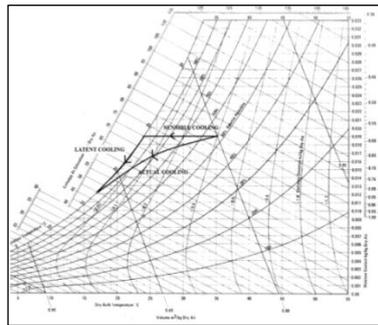
Figure 2. Dehumidification process on psychrometric chart
