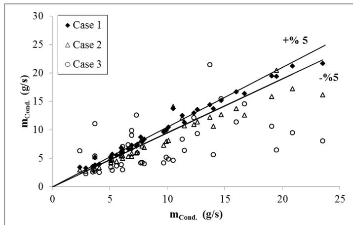
**Figure 5.** Comparison of condensate rate obtained from the model with simulation results
