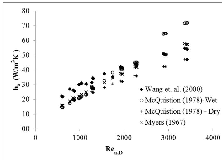
**Figure 6.** Comparison of heat transfer coefficients obtained from correlations
