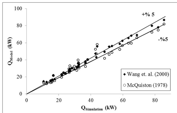
**Figure 7.** Comparison of the heat capacity rates based on Wang et. al. (2000) and McQuiston (1978) correlations
