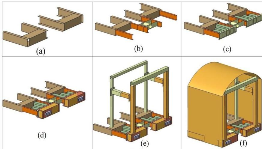
**Figure 3.** Crush zone component and integration sequence for the passenger wagon.
