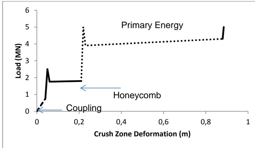
**Figure 1.** Ideal crush zone deformation-load curve.
