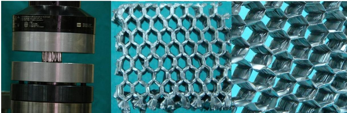
**Figure 6.** Quasi-static crush test of aluminum alloy honeycomb specimens in out-of-plane direction.
