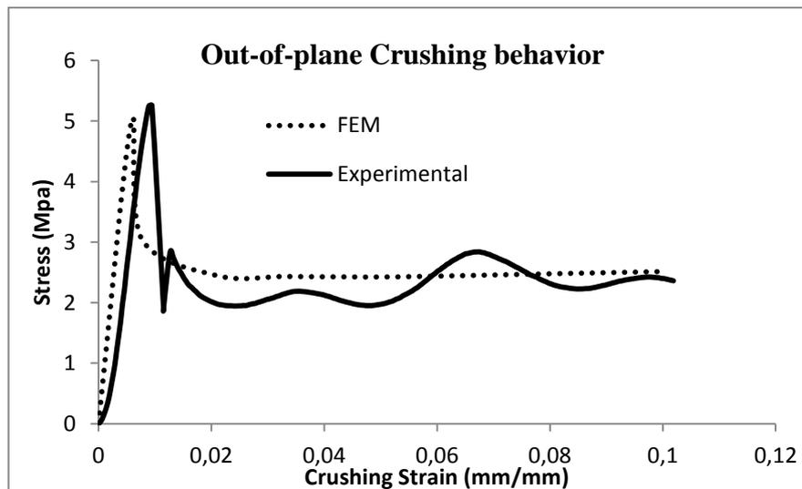
**Figure 4.** Crushing strain-stress for out-of-plane crushing behavior of the honeycomb structure.
