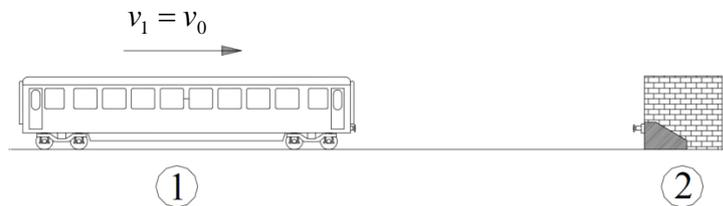
**Figure 2.** One wagon impacts into a rigid standing wall.
