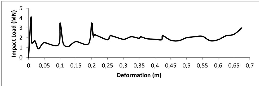
**Figure 8.** Crushing behavior of primary energy absorber component in crush zone.
