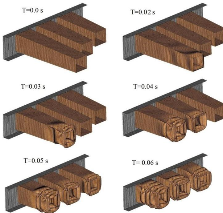
**Figure 9.** Plastic deformation of primary energy absorber component at different instants.
