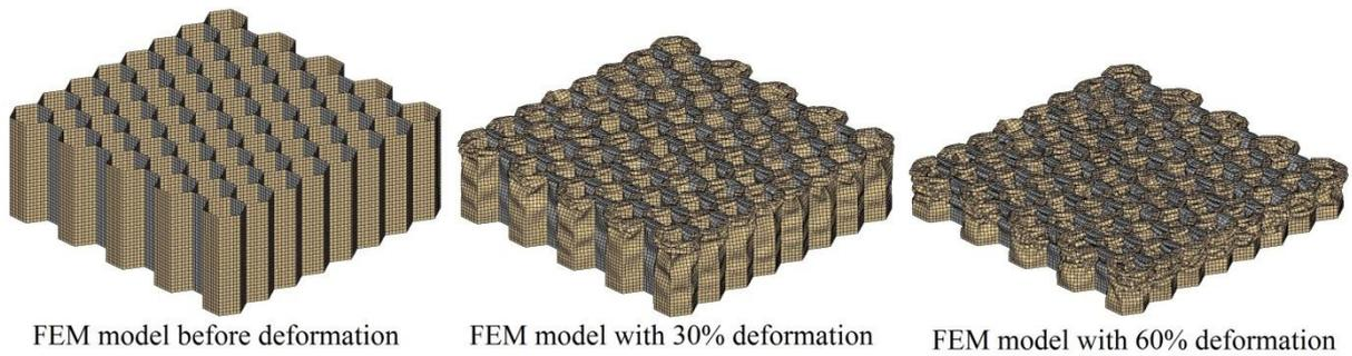
**Figure 5.** FE deformation stages of aluminum alloy honeycomb specimens in out-of-plane direction.
