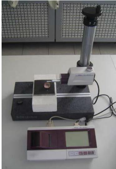
**Figure 3.** Mitutoyo SJ-401 surface profilometer
