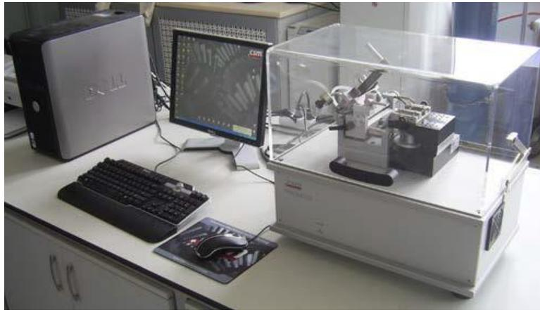
**Figure 1.** CSM tribometer
