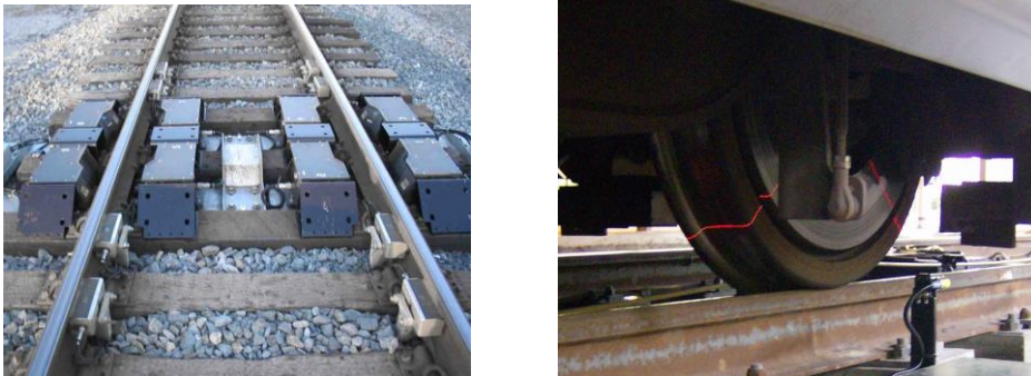
Figure 3. A view of wheel profile measurement(Web-1)
