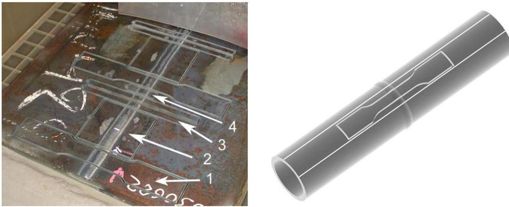
**Figure 5.** Extraction the weld sample (left), the cylindrical test sample image (right) [55].
