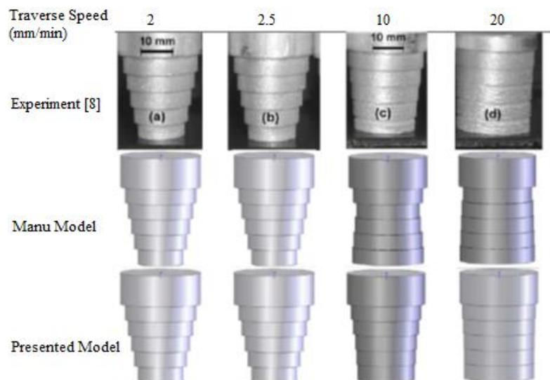
**Figure 12.** Comparison of experimental results with the Manu model [59].
