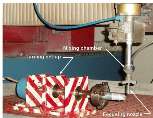
**Figure 7.** Turning experimental setup view [56].
