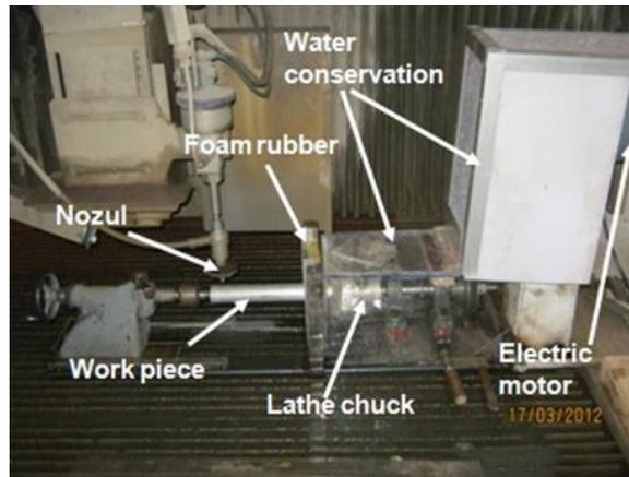
**Figure 13.** The image of Turning experimental setup [60].
