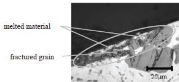
**Figure 2.** Cutting edge of the cutting tool consisting of chips formation of fractures SEM image. [53].
