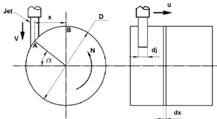
**Figure 6.** Water jet impact angle view [56].
