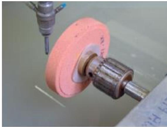
**Figure 3.** Experimental setup of textile grinding wheel turning mechanism. [54].
