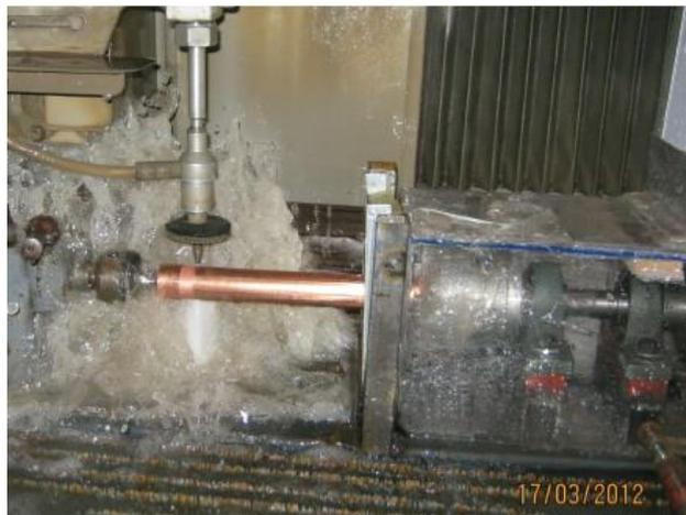
**Figure 14.** (Cu-Cr-Zr) alloy of copper with the turning of abrasive water jet [61].
