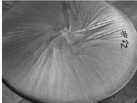
**Figure 10.** After the turning process image of a waviness of the center face [58].
