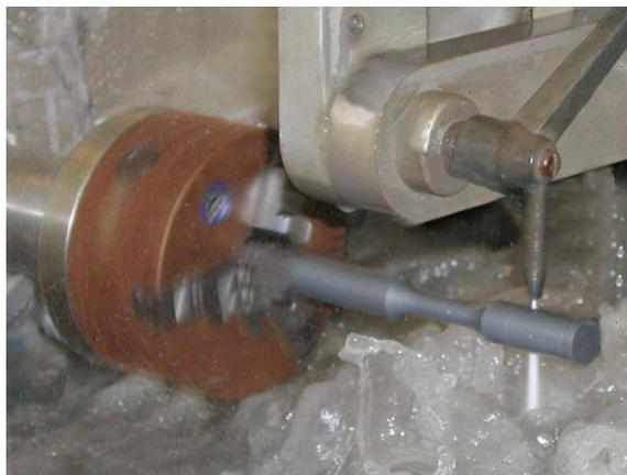
**Figure 4.** AWJ experimental setup with the turning. [55].
