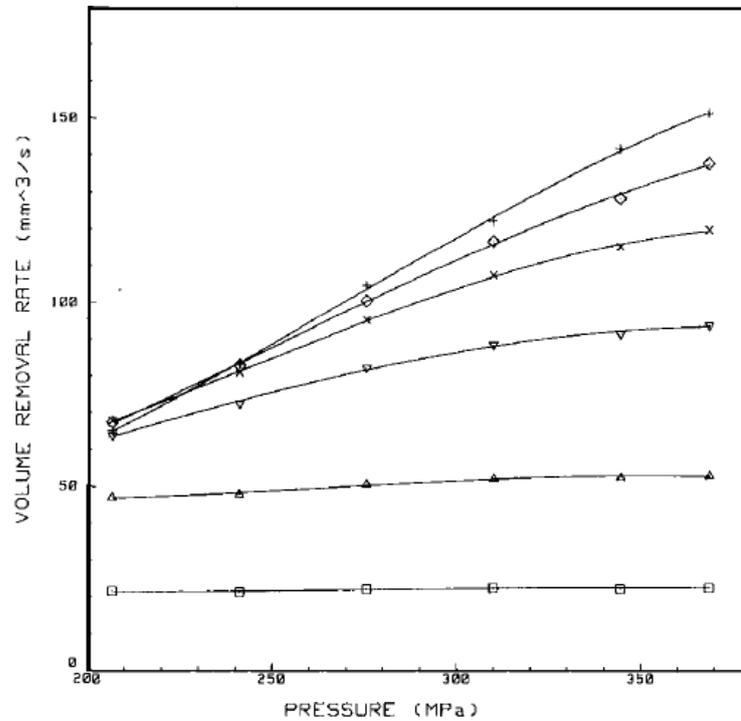
**Figure 8.** The amount of feed pump pressure and nozzle effect of the volume of material removal [57].
