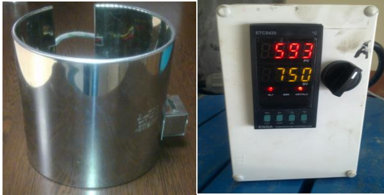
Figure 5. Heater resistance and heat control panel.
