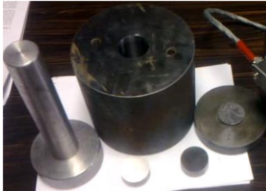
Figure 4. The mould elements which were grinded after heat treatment.
