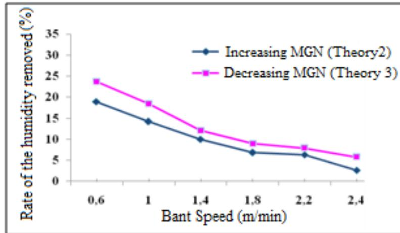
**Figure 3.** The change of the humidity removed according to the band speed with increasing and decreasing magnetron output power.
