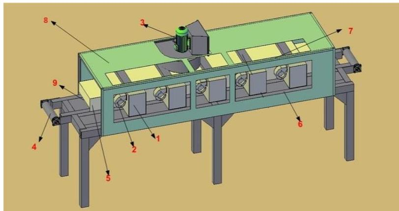
**Figure 1.** Specially manufactured MW oven with prototype conveyor. 1.Mikrowave generator (MGN, high voltage transformer and temperature control device), 2.MGN cooling fan, fan 3.Circulation fan, 4.Belt system 5.Stainless interior cabin, 6.Side shuttings 7.Top shuttings, 8.Stainless outer cabinet, 9.Entry point.
