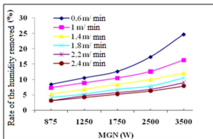
Figure 2. With different band speeds, depending on the strength of MGN, the change in humidity rate.
